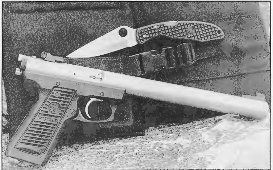
The Operator Pak, designed for government operatives, consists of a highly sophisticated sound-suppressed Ruger 22/45 pistol with a unique bolt lock, a proprietary-size Safepacker holster and a Spyderco Clipit Endura locking folder knife.
